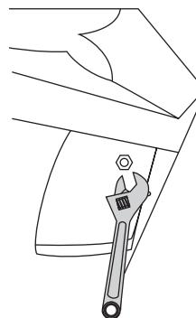
After tightening, ensure that there is no gap between the appliance and the wall. If so, use sealant to fill the gap.
