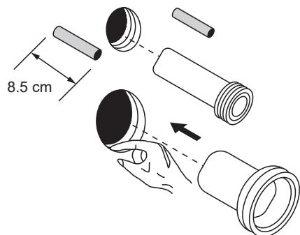
Fix the closet in the rag-bolts and insert the washers and nuts.
